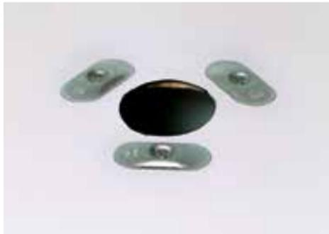
Mechanically fix the membrane around the outlet to the decking with fixing plates and screws.
