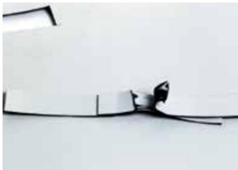
The membrane must fail outside the welding seam.
