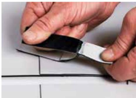
Check the sample weld with a destructive test (see 14.2 page 55).
