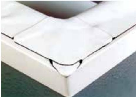
Spot-weld, pre-weld and weld the patch onto the corner.
