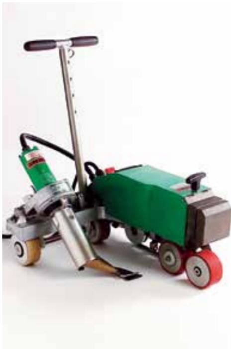
Using automatic welding equipment such as the Varimat Leister equipped with a TEXSA SCRAPER NOZZLE.
